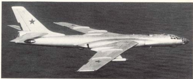
The Badger-F is fitted with two underwing pods supposedly connected with targeting of Shaddock class cruise missiles.
