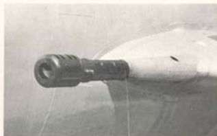
Above: a Czech Air Force Farmer-C. Below: the protruding left wing Nudelmann-Richter NR-30 30 mm cannon.
