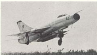
Above: the Su-11 (Fishpot-C) with two Anab AAM missiles. Below: the previous version (Su-9 Fishpot-B) with pylons for four older Alkali AAM.
