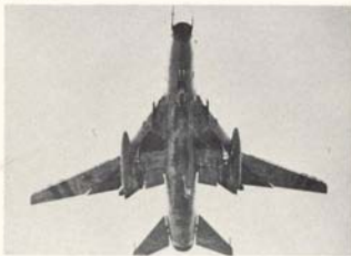
The series production Su-17 has four fuselage hardpoints.
