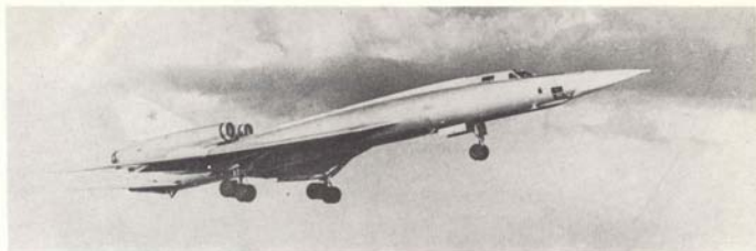
The very first version of the Tu-22 (Blinder-A), without in-flight refuelling capability and with free-fall only bomb bay.
