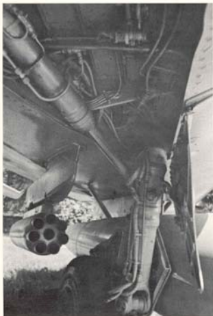
The starboard mainwheel housing and an UV-7-57 55 mm light rocket launcher in a Czech Farmer-C.
